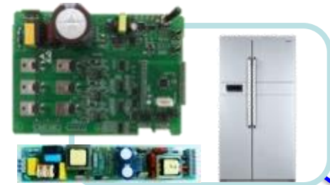
Refrigerator SMPS + Inverter
